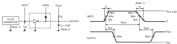
Note 1: Pulse Width 50  $\mu$ s, Duty Cycle 10% Output Impedance 50  $\Omega$ , t<sub>f</sub> ≤ 5ns, t<sub>f</sub> ≤ 10 ns Note 2: C<sub>L</sub> includes probe and jig capacitance
